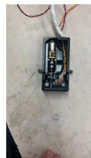
A hand-held device with exterior features similar to a pulse oximeter that applies a certain force to the fingernail, and measures CRT with a photoresistor.
