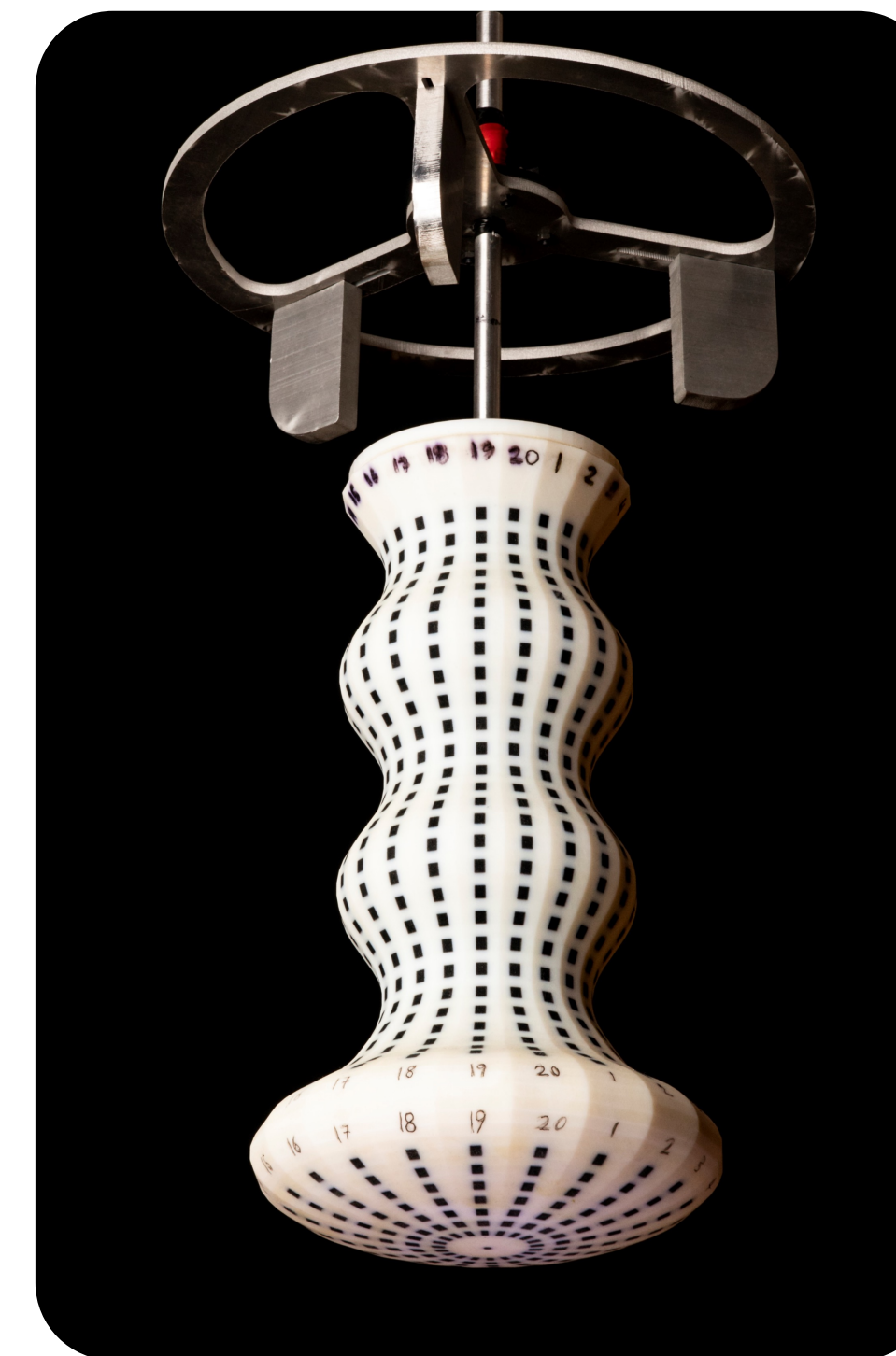
The calibration object allows for simultaneous stereo calibration for each camera. It features 700 black rectangular planar faces on a white background. The 3D coordinates of the centroids of black dots used to obtain the stereo triangulation parameters
